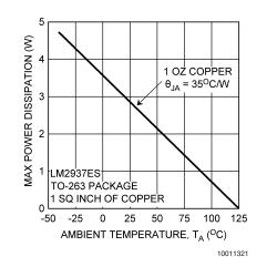
FIGURE 4. Maximum Power Dissipation vs  $\rm T_{AMB}$  for the TO-263 Package
