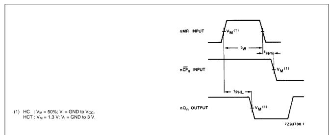
Fig.7 Waveforms showing the master reset (nMR) pulse width, the master reset to output (nQ<sub>n</sub>) propagation delays and the master reset to clock (n $\overline{CP}_n$ ) removal time.
